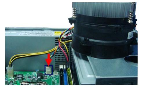
2. Position the heat sink fan assembly on top of the processor, making sure the screws are aligned with the screw holes on the main board.
